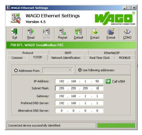
Now you can set the IP-address and the subnet mask of your Ethernet Controller in accordance with the settings of your local network. To connect to the World Wide Web, the controller uses the router (IP of the router) as gateway and DNS-server. After changing the described settings, save them with [Write] into your Ethernet Controller.
