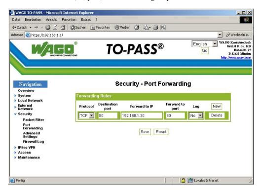
To communicate with a Web-Portal it is necessary to forward port 80 of the incoming data to port 80 of the local application.
