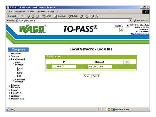
The router is able to work as a DHCP-server to assign addresses automatically. This function is disabled in the described application. Therefore the other network devices of the routers local network (PC and WAGO Ethernet Controller) have constant IP-addresses.
