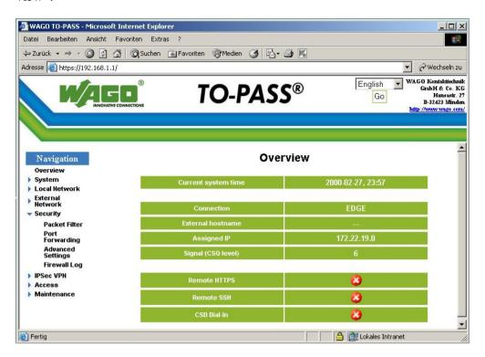
The value "CSD Dial-In" should be greater than 11. In addition you can check the IP of your router in the external network.
