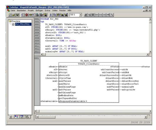
The function block handles the communication between Ethernet Controller and Web-Portal and provides information about the actual connection.
