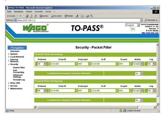
Incoming: With these settings you can set the rules for incoming IP-packets. Data source is the sender of the IP-packets. Aim of data is the IP-address of the local application (Ethernet Controller). If you choose "0.0.0.0/0" and "ANY", data from any addresses can pass by. The firewall is deactivated.
